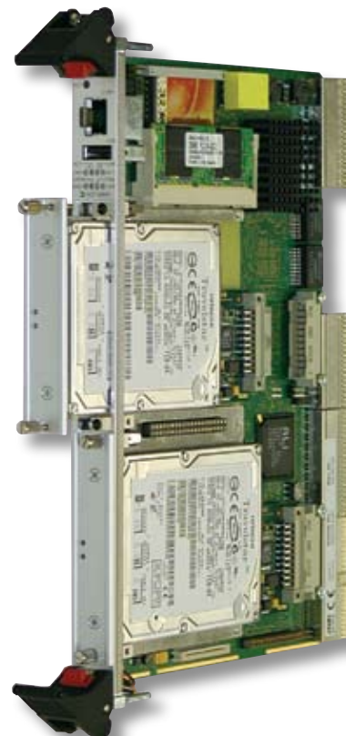
Figure 3 NAS blade showing dual drive shuttles.
