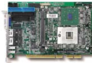
Half-Size Low Power SBC with Dual GbE, LVDS & CF
