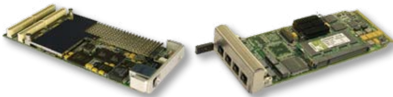
Figure 1 The PMC standard (left) provides a platform for modular computing. The recently ratified AMC standard (right) takes modular multiprocessing to a new level, while retaining a similar form-factor.
