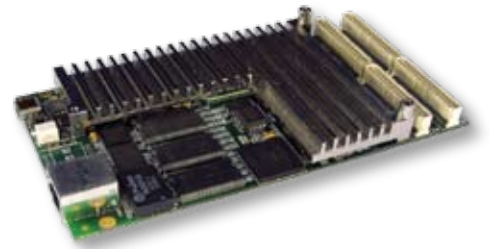
Figure 3 SMP Processor PMC modules require a novel approach to cooling. XPedite6200 utilizes a heat sink that covers both CPUs and the system controller.
