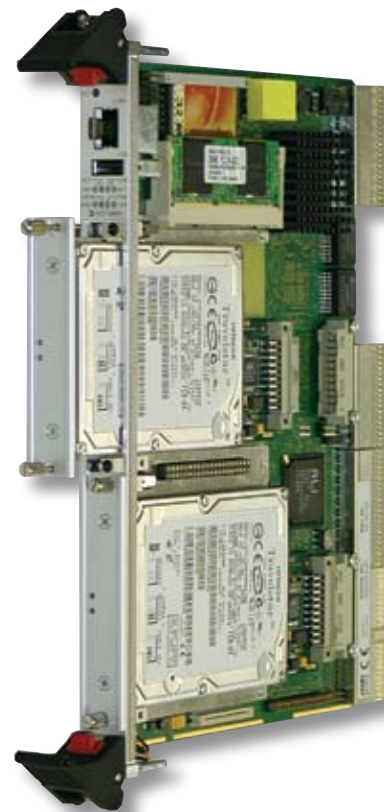
Figure 3 NAS blade showing dual drive shuttles.
