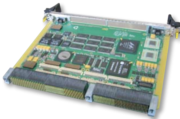
Figure 4 Example of a VITA 46 single board computer from Curtiss-Wright, which features high-speed MultiGig RT interface and high-speed XMC connectors.
