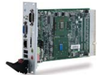
3U CompactPCI CPU Module with Dual GbE & USB 2.0
