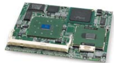
ETX Module with High-End Graphics & Optional HDTV I/F
