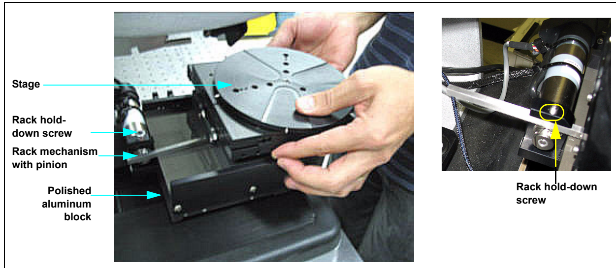
Figure 2-21: Placing the Stage on the Polished Aluminum Block
