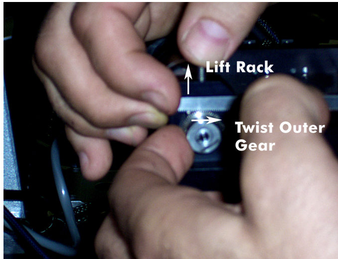
Figure 2-23: Adjusting the Anti-Backlash Gear Mechanism
