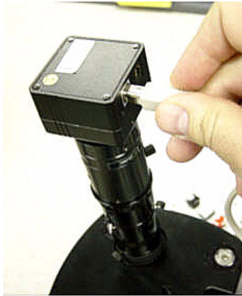
Figure 2-19: Plugging the USB Cable into the Camera
