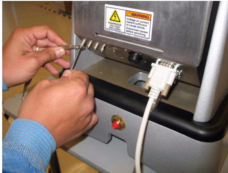
Figure 2-15: Connecting the Ground Strap
