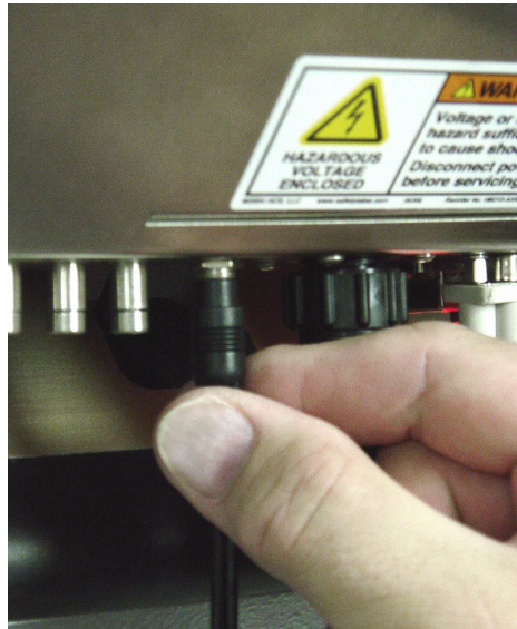
Figure 2-13: Connecting the Power Supply Cable
