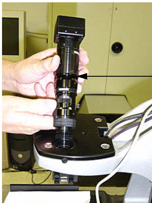
Figure 2-18: Screwing the Optical Assembly into the Optics Mounting Plate
