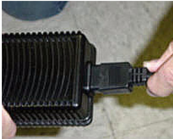
Figure 2-14: Connecting the AC Power Cord to the Power Supply
